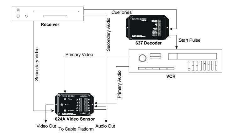
Normal program video and audio are fed to your cable platform through the 624A Video Sensor. When a correct 'START' cue tone sequence is received a START pulse is sent to the VCR. When the VCR starts to produce a video signal, the video sensor will switch to the primary input. When the VCR's video stops the video sensor switches back to the normal program on the secondary connections.
